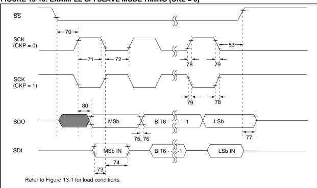
FIGURE 13-10: EXAMPLE SPI SLAVE MODE TIMING (CKE = 0)
