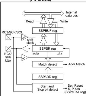
The SSP module has five registers for  $I^2C$  operation. These are the:
