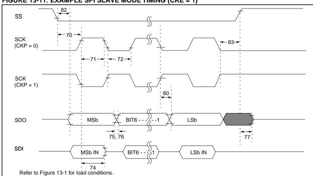
FIGURE 13-11: EXAMPLE SPI SLAVE MODE TIMING (CKE = 1)
