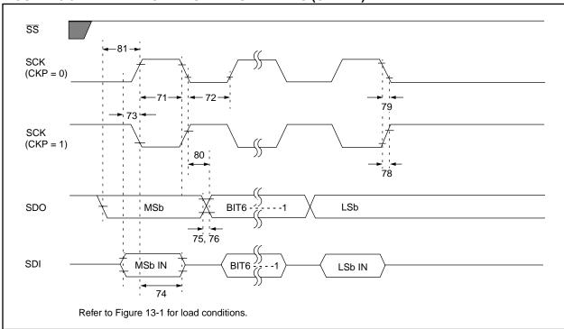
FIGURE 13-9: EXAMPLE SPI MASTER MODE TIMING (CKE = 1)
