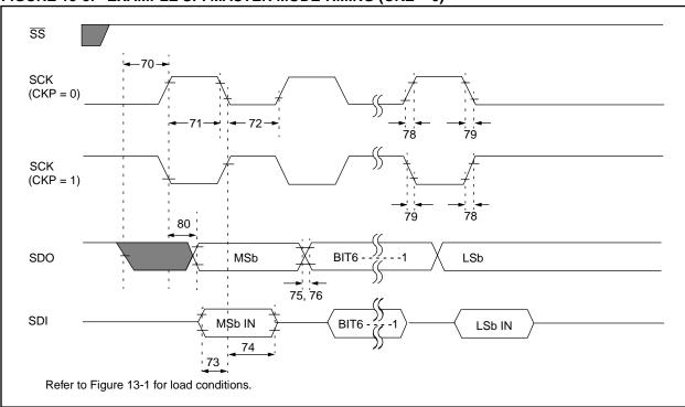
FIGURE 13-8: EXAMPLE SPI MASTER MODE TIMING (CKE = 0)
