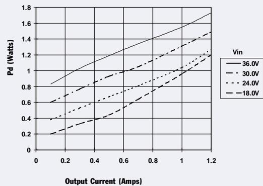
Note A: All data listed in the above graphs, except for derating data, has been developed from actual products tested at 25°C. This data is considered typical data for the isolated DC-DC converter.
