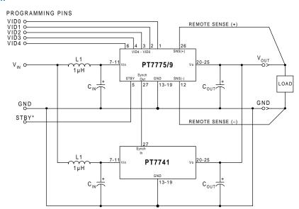
External Capacitors: When used with a PT7779, the PT7741 requires a minimum outur capacitance of 330µF. The maximum allowable output capacitance is 30,000µF. The PT7741 also requires a minimum input capacitance of 2400µF, which must be rated for a minimum of 2.0Arms of ripple current. For transient or dynamic load applications, additional capacitance may be required. For further information, see the accompanying application note on capacitor selection for this product.
