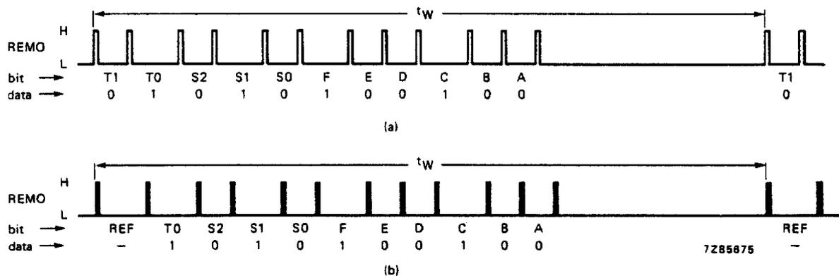
REF = reference time; T0 and T1 = toggle bits; S0, S1 and S2 = system address; A, B, C, D, E and F = command bits
