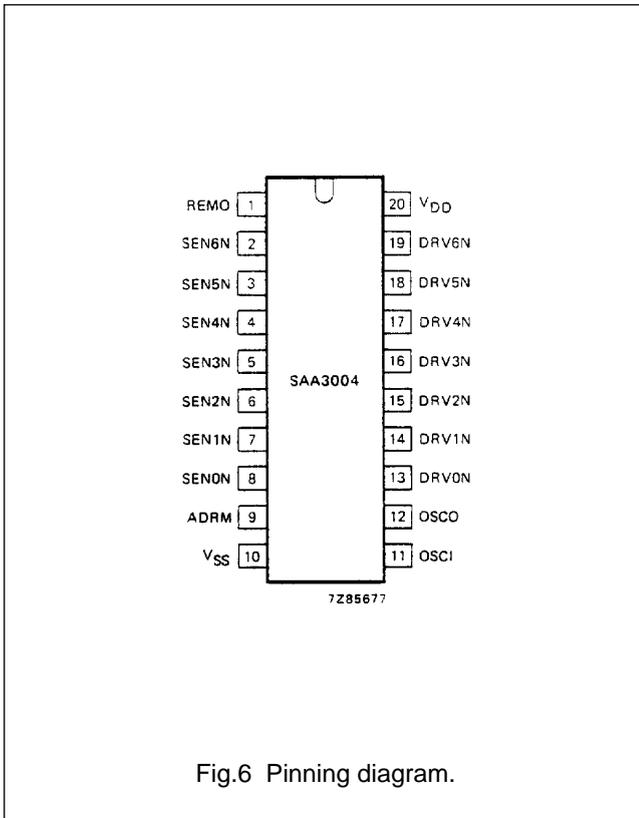
Fig.6 Pinning diagram.
