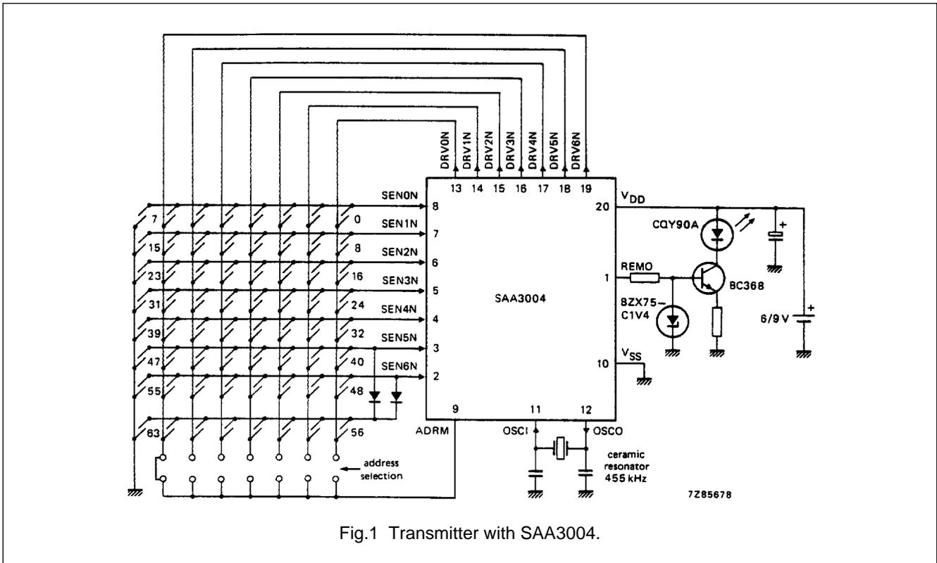
Fig.1 Transmitter with SAA3004.
