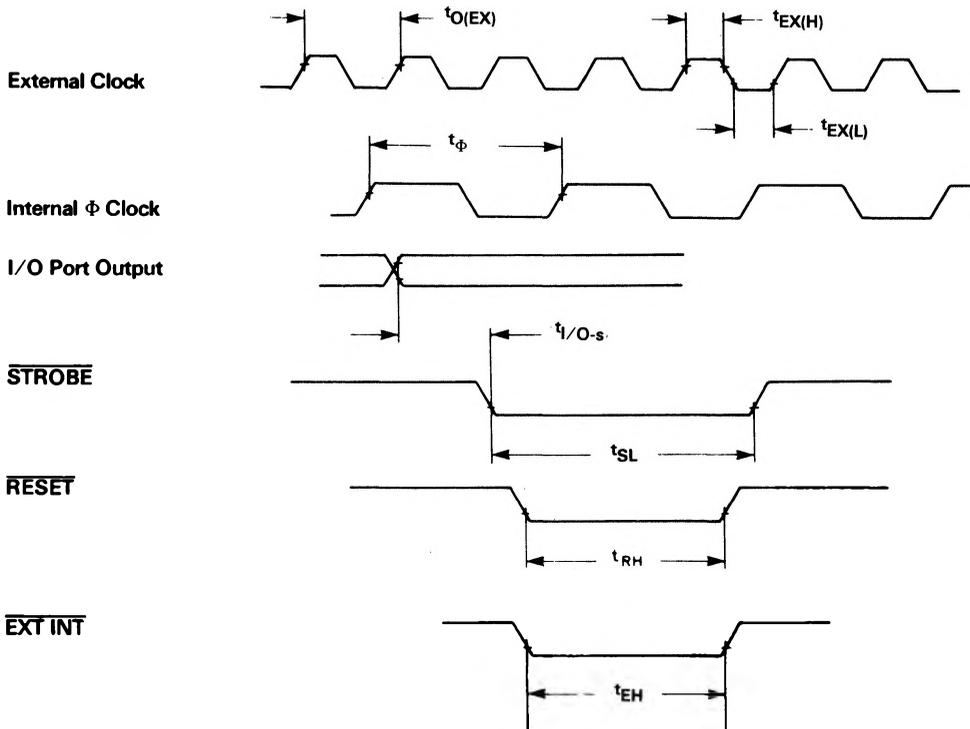
Note: All AC measurements are referenced to  $V_{IL}$  max.,  $V_{IH}$  min.,  $V_{OL}$  (.8v), or  $V_{OH}$  (2.0v).
