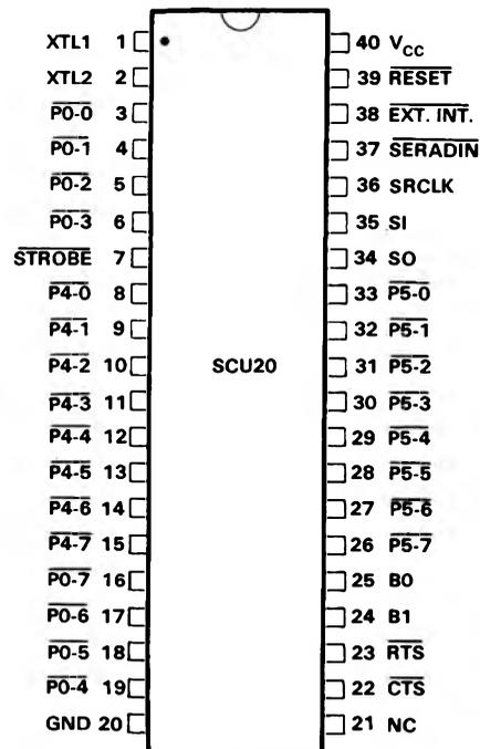
The SCU20 can be used for both monitoring and control systems where remote intelligence is required. It can be configured to provide many different input/output and data acquisition functions through its 24 I/O pins. Such intelligent functions as Data Log and Event Counters allow many different applications that will not burden the host system with constant update requirements.
