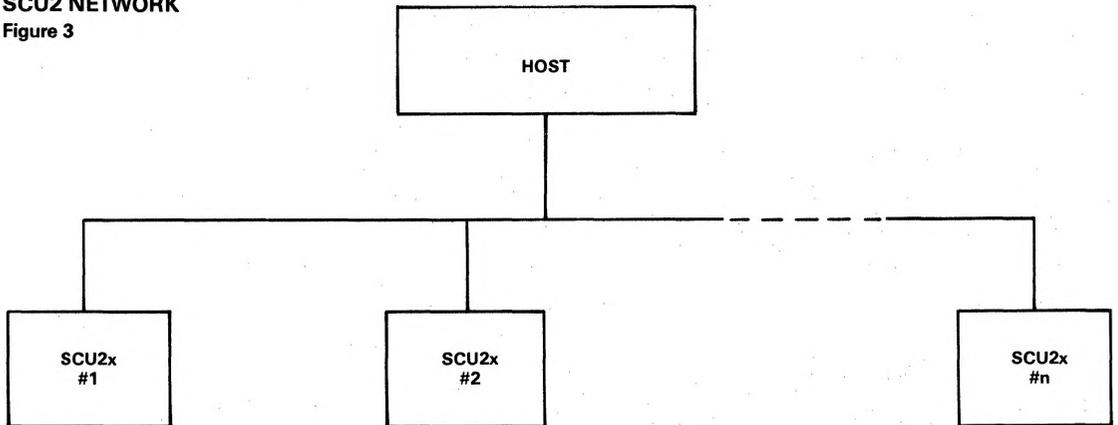
Each SCU2x in the network has an individual address to which it will respond. All SCU2x devices in the network are slave processors to the host, and are unable to initiate communications except in response to the host.
