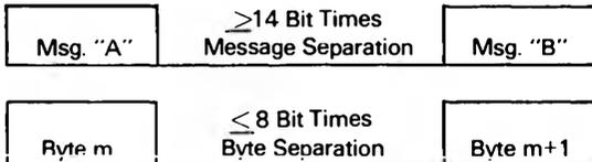
Messages are to be transmitted in block mode, with a message separation of at least 14 bit times. Interbyte separations should be no more than 8 bit times within a message.
