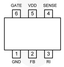
Figure 4. SOT Pin Configuration (Top View)
