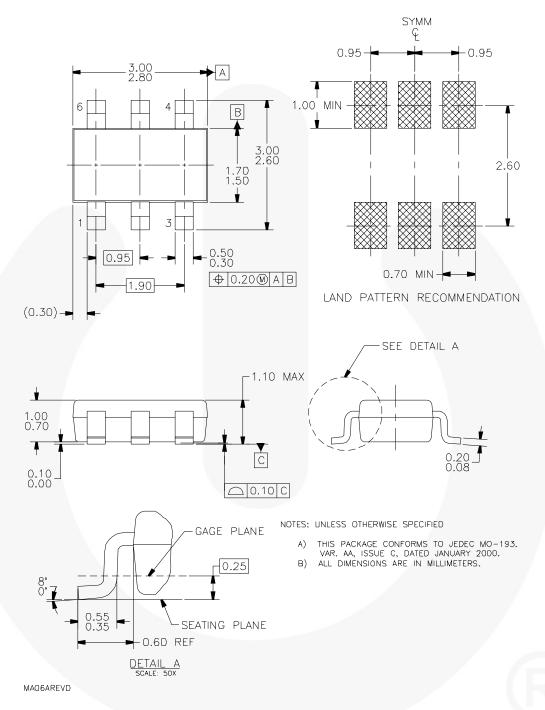
Figure 15. 6-Pin SSOT-6 Package
