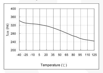
Figure 14. t<sub>LEB</sub> vs. T<sub>A</sub>
