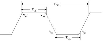
Figure 1. Clock Cycle/High/Low Times
