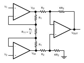
Figure 42. Instrumentation Amplifier
