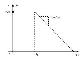
Figure 45. Lowpass Filter Transfer Function
