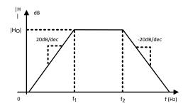
Figure 49. Bandpass filter Transfer Function
