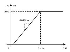
Figure 47. Highpass Filter Transfer Function
