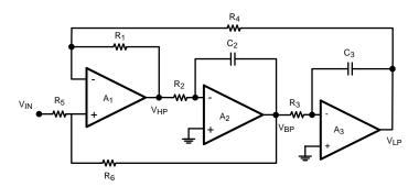
Figure 50. State Variable Active Filter
