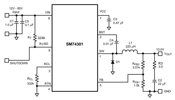
Figure 12. SM74301 Example Circuit
