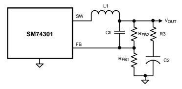
Figure 15. Reduced Ripple Configuration
