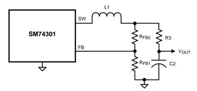
Figure 17. Alternate Minimum Output Ripple
