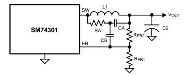
Figure 16. Minimum Output Ripple Using Ripple Injection
