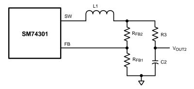
Figure 9. Low Ripple Output Configuration
