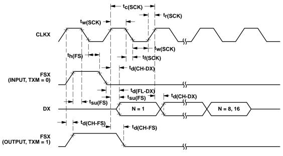
Figure 15. Serial Port Transmit Timing
