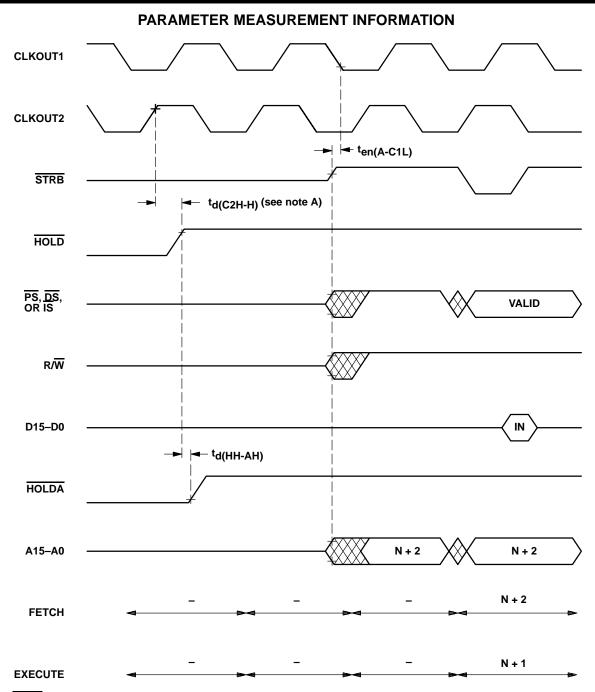
NOTE A: HOLD is an asynchronous input that can occur at any time during a clock cycle. If the specified timing is met, the exact sequence shown will occur; otherwise, a delay of one CLKOUT2 cycle will occur.
