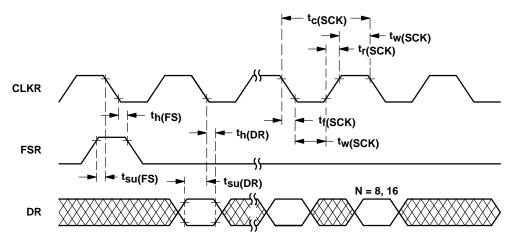
Figure 14. Serial Port Receive Timing
