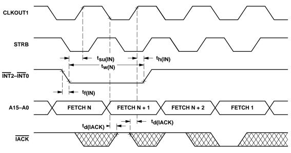
Figure 9. Interrupt Timing
