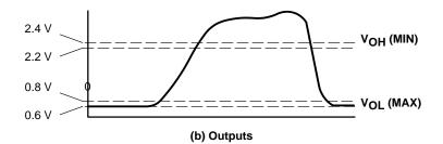
Figure 3. Voltage Reference Levels
