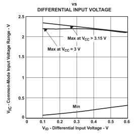
Figure 1.  $V_{IC}$  Versus  $V_{ID}$  and  $V_{CC}$
