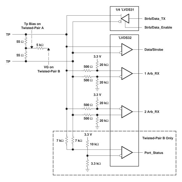
NOTES: A. Resistors are leadless, thick film (0603), 5% tolerance.
