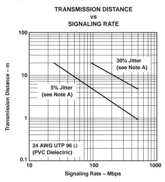
A. This parameter is the percentage of distortion of the unit interval (UI) with a pseudorandom data pattern.
