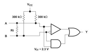
Figure 16. Open-Circuit Fail-Safe of LVDS Receiver
