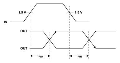
Figure 2. Output Propagation Delay
