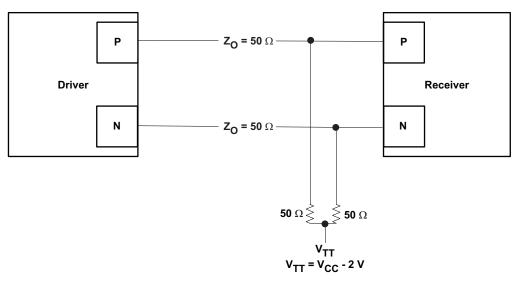
Figure 1. Termination for Output Driver
