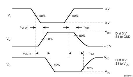
Figure 7. Measurement of Receiver Enable/Disable Times With Driver Enabled
