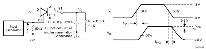
NOTE: D at 3 V to test non-inverting output, D at 0 V to test inverting output.
