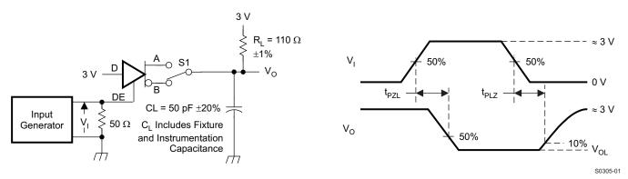
NOTE: D at 0 V to test non-inverting output, D at 3 V to test inverting output.
