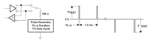
Figure 16. Test Circuit and Waveforms, Transient Overvoltage Test
