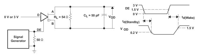
Figure 8. Driver Standby/Wake Test Circuit and Waveforms
