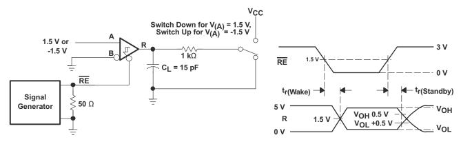
Figure 14. Receiver Standby and Wake Test Circuit and Waveforms
