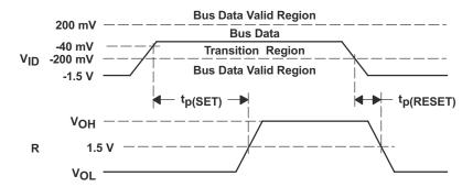
Figure 15. Receiver Active Failsafe Definitions and Waveforms
