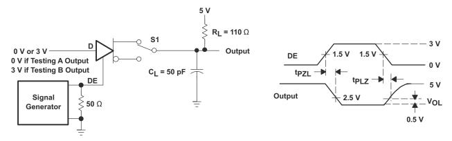
Figure 7. Driver Enable/Disable Test, Low Output
