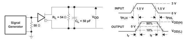
Figure 3. Driver Switching Test Circuit and Waveforms
