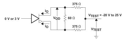
Figure 2. Driver Test Circuit, VoD With Common-Mode Loading
