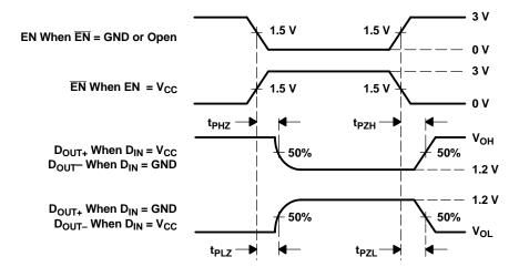
Figure 5. Driver 3-State Delay Waveform
