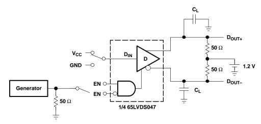
Figure 4. Driver 3-State Delay Test Circuit
