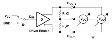
Figure 1. Driver V<sub>OD</sub> and V<sub>OC</sub> Test Circuit
