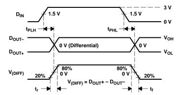
Figure 3. Driver Propagation Delay and Transition Time Waveforms
