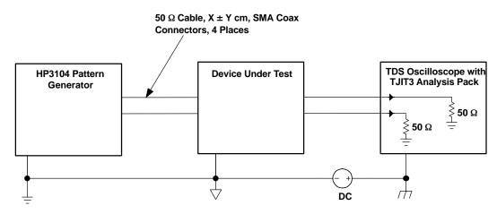
Figure 5. Jitter Measurement Setup
