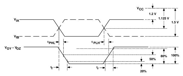
Figure 4. Propagation Delay and Transition Time Test Waveforms
