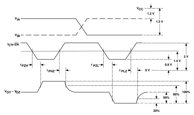
Figure 6. Enable and Disable Time Test Waveforms
