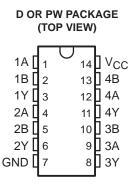
The 'AHCT00 device performs the Boolean function  $Y = \overline{A \bullet B}$  or  $Y = \overline{A} + \overline{B}$  in positive logic.
