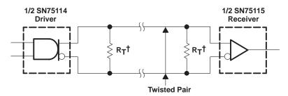
$<sup>^{\</sup>dagger}$  R<sub>T</sub> = Z<sub>O</sub>. A capacitor can be connected in series with R<sub>T</sub> to reduce power dissipation.
