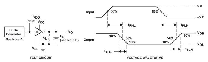
NOTES: A. The pulse generator has the following characteristics:  $t_W$  = 25  $\mu$ s, PRR = 20 kHz,  $Z_O$  = 50  $\Omega$ ,  $t_f$  =  $t_f$  < 50 ns.
