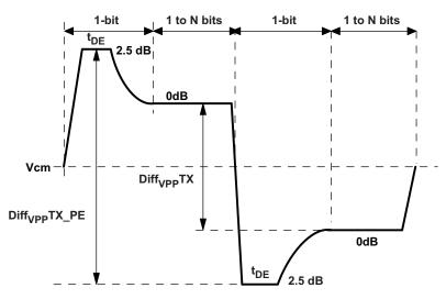
Figure 6. TX Differential Output with 2.5 dB Pre-Emphasis Step
