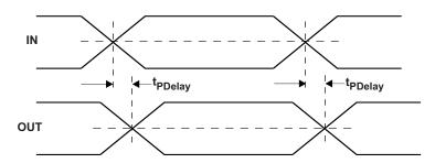
Figure 4. Propagation Delay Timing Diagram
