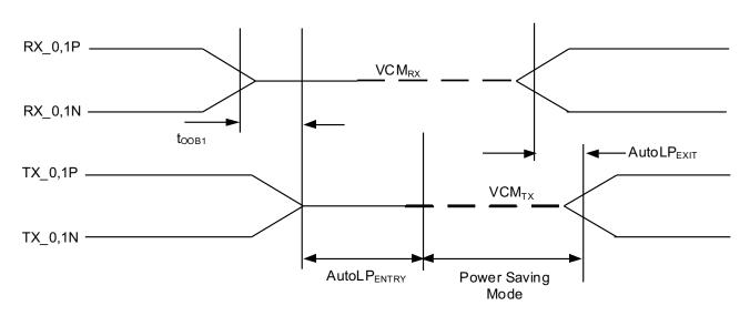
Figure 7. Auto Low Power Mode Timing
