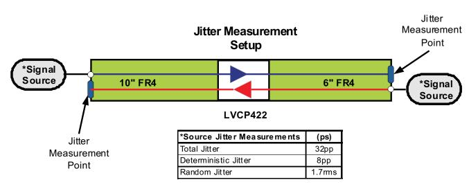
Figure 2. Output Jitter Measurement Test Setup
