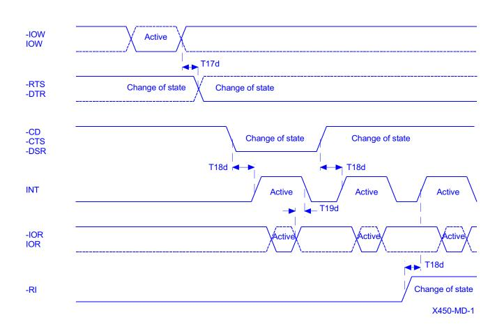
Modem input/output timing
