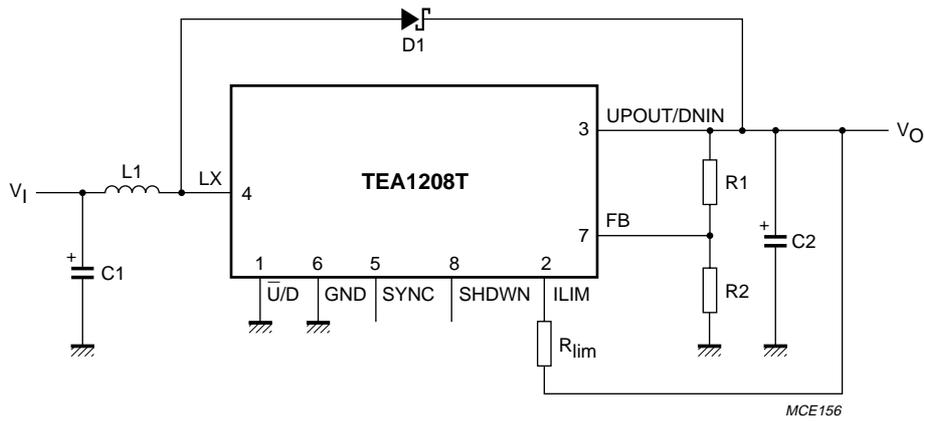
Fig.5 Complete application diagram for up conversion.
