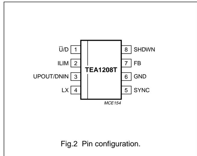
Fig.2 Pin configuration.
