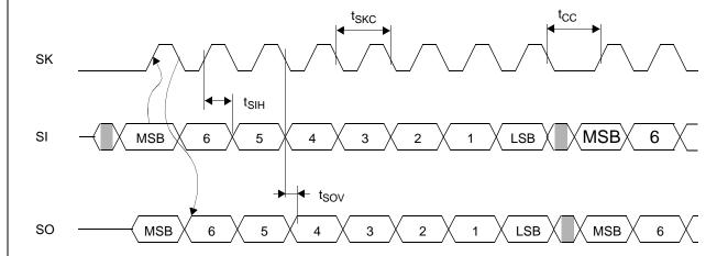
NOTE: The first eight SK cycles shift out the current contents of the shift register.
