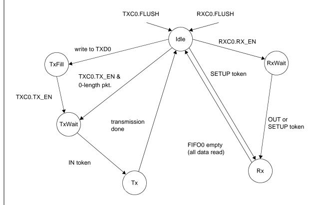
Figure 16. Endpoint 0 Operation
