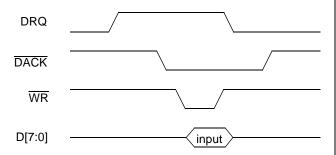
Figure 8. DMA Write to USBN9602
