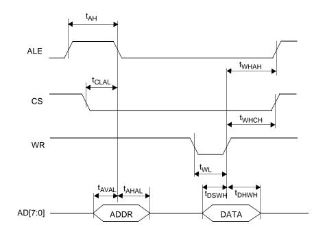
Figure 25. Multiplexed Mode Interface Write Timing
