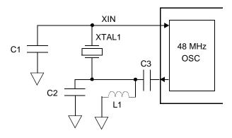
Figure 2. 3rd Harmonic Crystal Oscillator Connections
