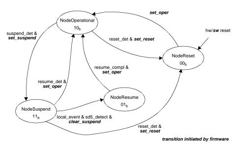
Figure 14. Node Functional State Diagram
