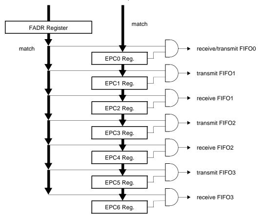
Figure 15. USB Function Address/Endpoint Decoding
