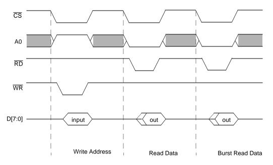
Figure 4. Non-Multiplexed Mode Basic Timing Diagram
