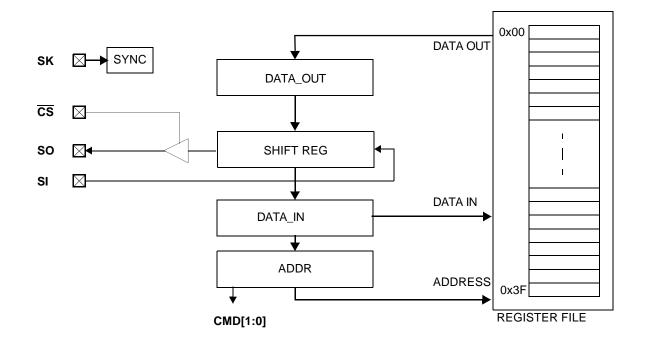
Figure 10. MICROWIRE Interface Block Diagram
