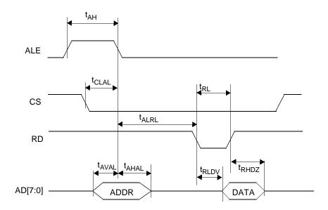
Figure 24. Multiplexed Mode Interface Read Timing
