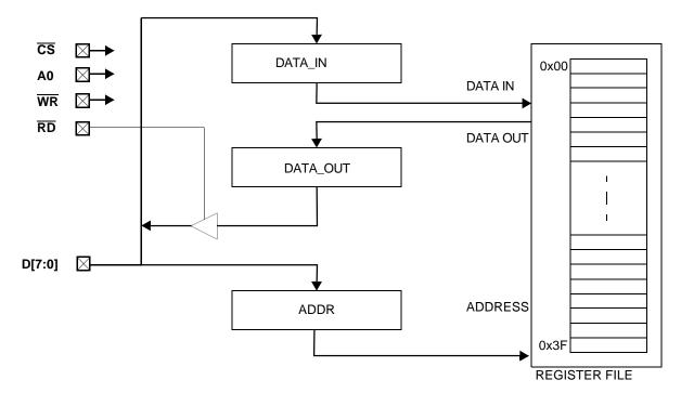
Figure 3. Non-Multiplexed Mode Interface Block Diagram
