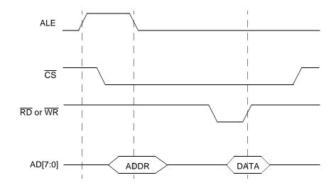
Figure 7. Multiplexed Mode Basic Read/Write Timing
