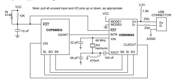
Figure 20. MICROWIRE Serial Interface
