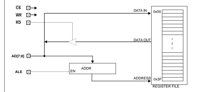
Figure 6. Multiplexed Mode Interface Block Diagram
