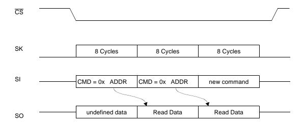
Figure 11. MICROWIRE Interface Basic Read Timing
