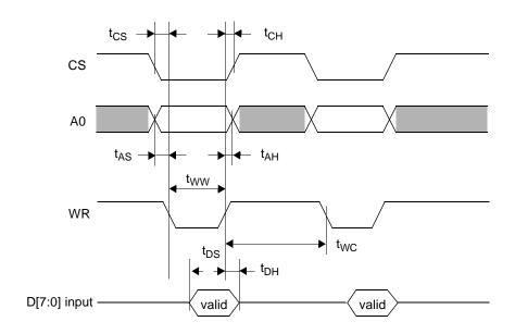
Figure 23. Non-Multiplexed Mode Write Timing
