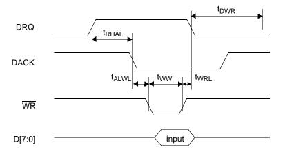
Figure 26. DMA Write to USBN9602
