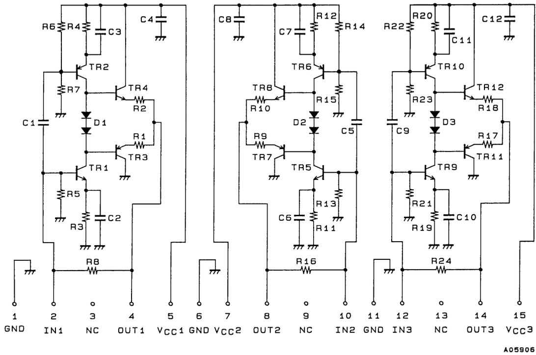
Test Circuit (for a single channel)
