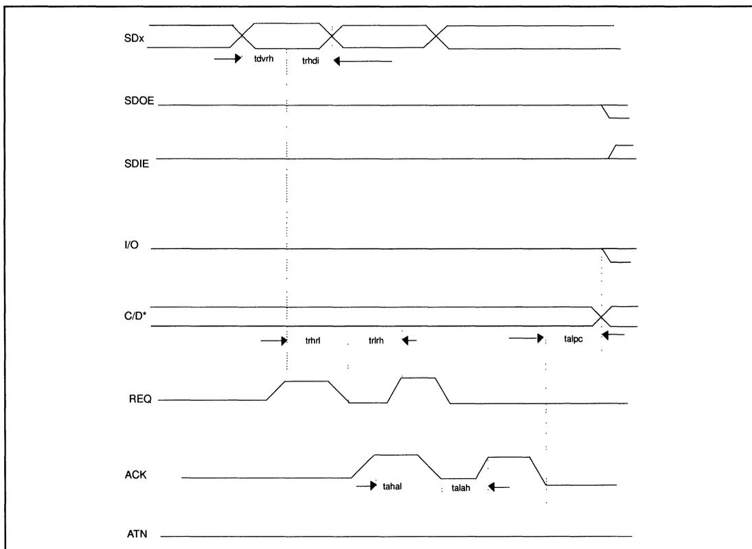
FIGURE 27. SYNCHRONOUS INFORMATION TRANSFER IN (T) TIMING
