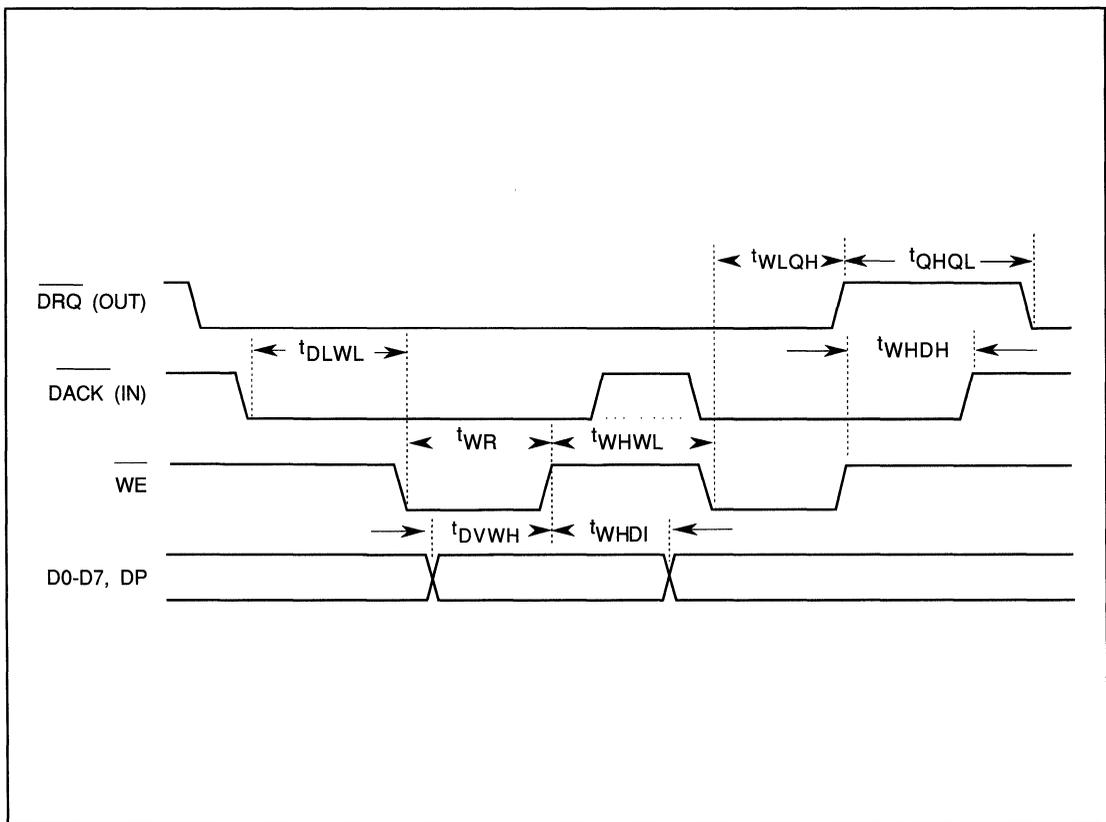
FIGURE 14. BURST DMA WRITE TIMING
