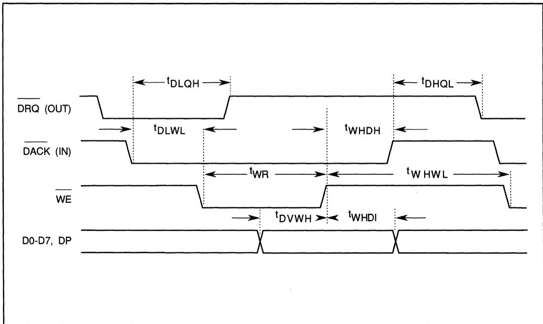
FIGURE 10. DMA WRITE
