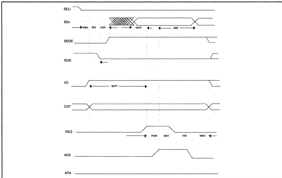
FIGURE 23. ASYNCHRONOUS INFORMATION TRANSFER IN (T) TIMING
