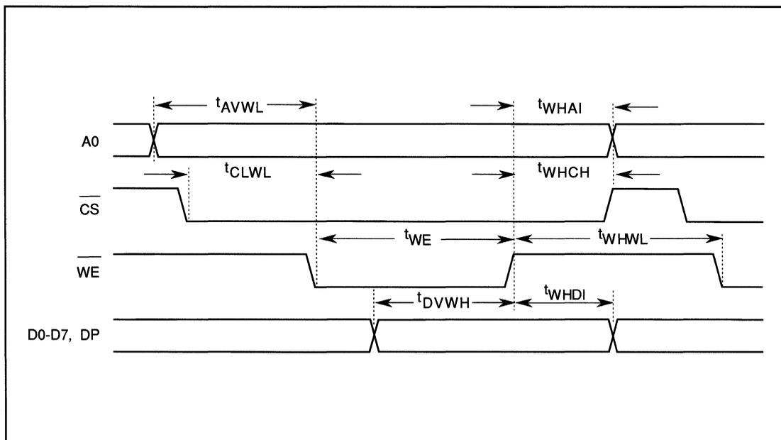
FIGURE 6. PROCESOR WRITE (INDIRECT ADDRESSING) TIMING
