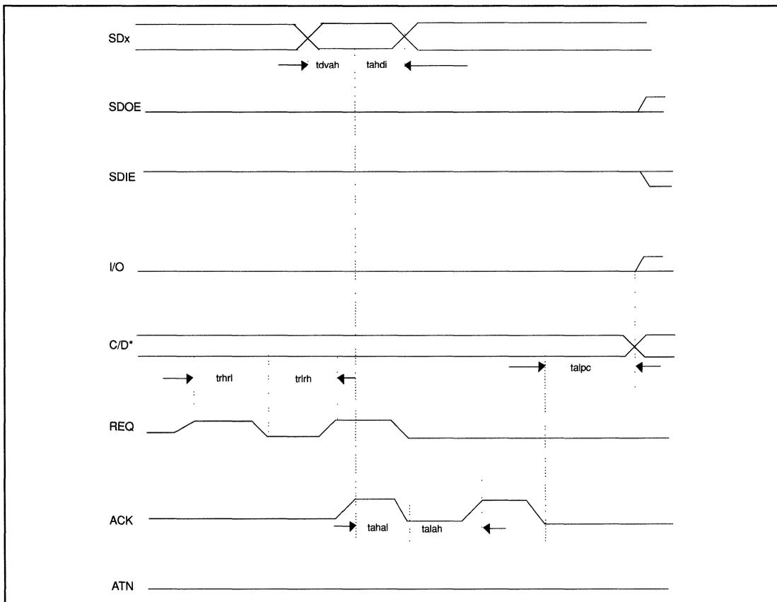
FIGURE 29. SYNCHRONOUS INFORMATION TRANSFER OUT (T) TIMING
