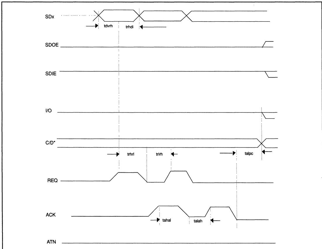
FIGURE 26. SYNCHRONOUS INFORMATION TRANSFER IN (I) TIMING
