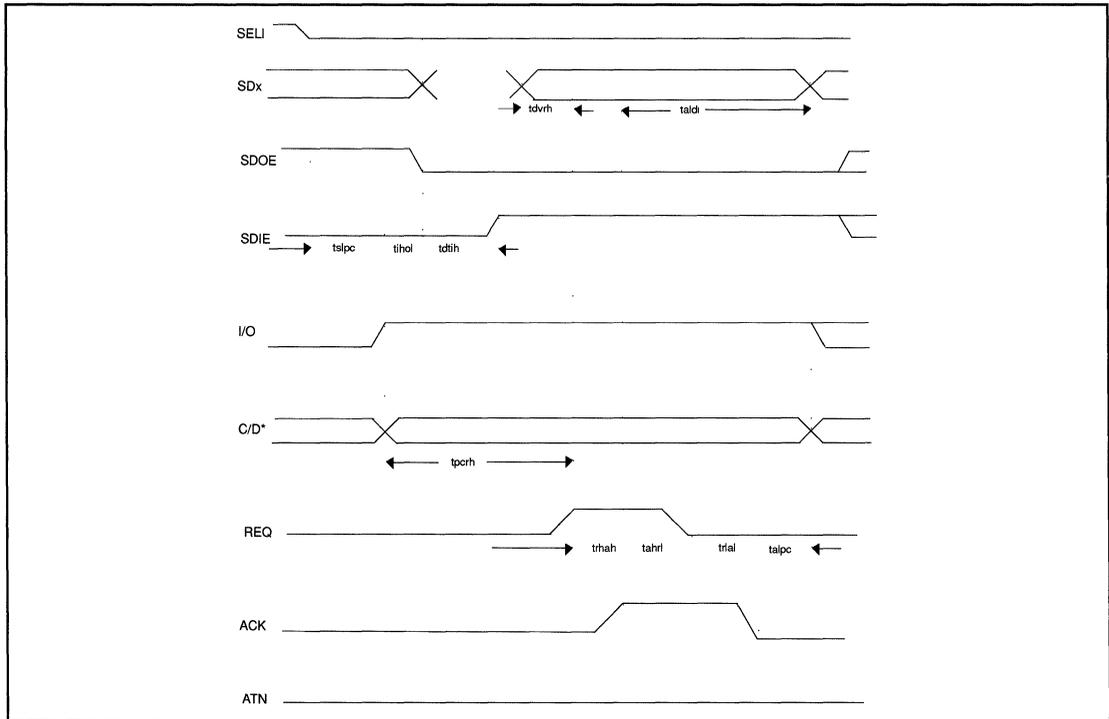
FIGURE 22. ASYNCHRONOUS INFORMATION TRANSFER IN (I) TIMING
