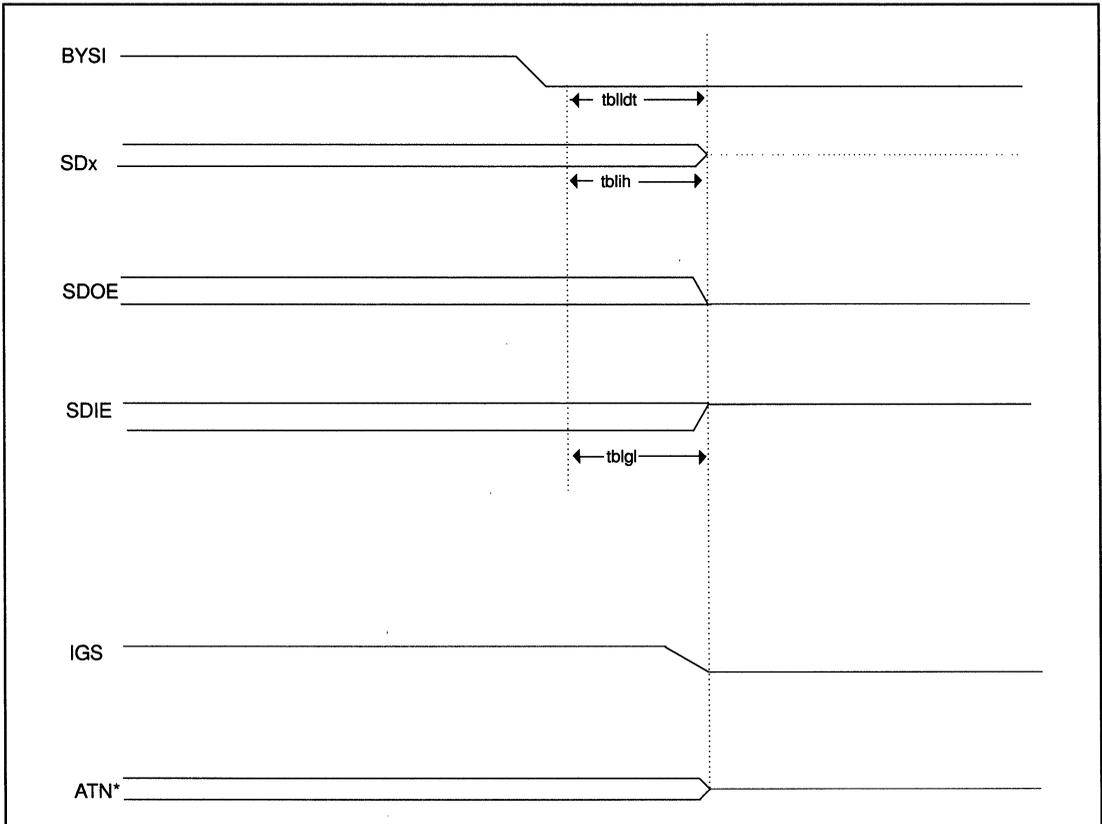
FIGURE 32. CONNECTED-AS AN-INITIATOR TO BUS FREE TIMING
