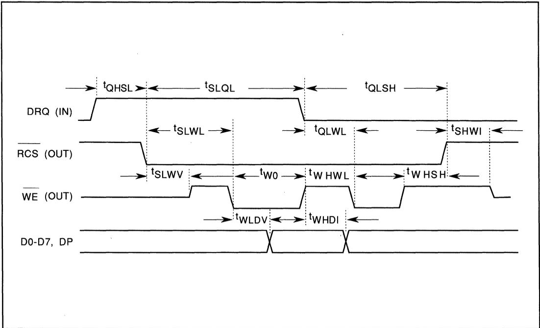
FIGURE 12. BUS BUFFER WRITE TIMING
