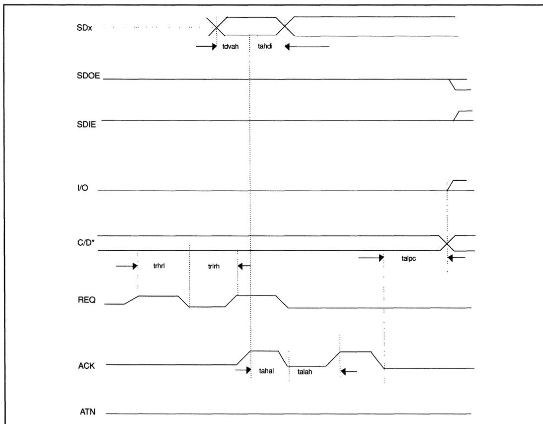
FIGURE 28. SYNCHRONOUS INFORMATION TRANSFER OUT (I) TIMING
