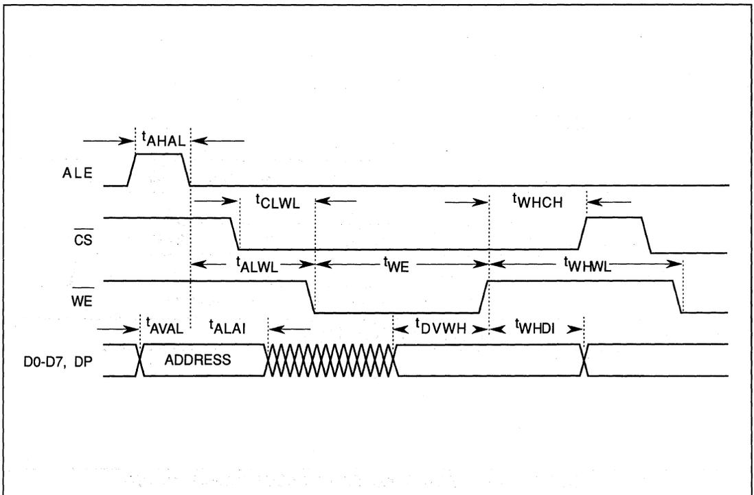
FIGURE 9-5. PROCESSOR WRITE (DIRECT ADDRESSING) TIMING
