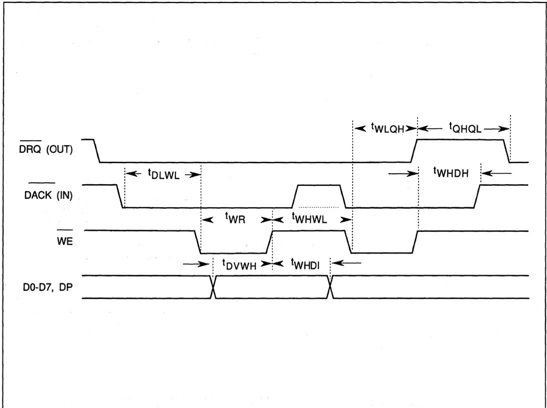
FIGURE 9-11. BURST DMA WRITE TIMING
