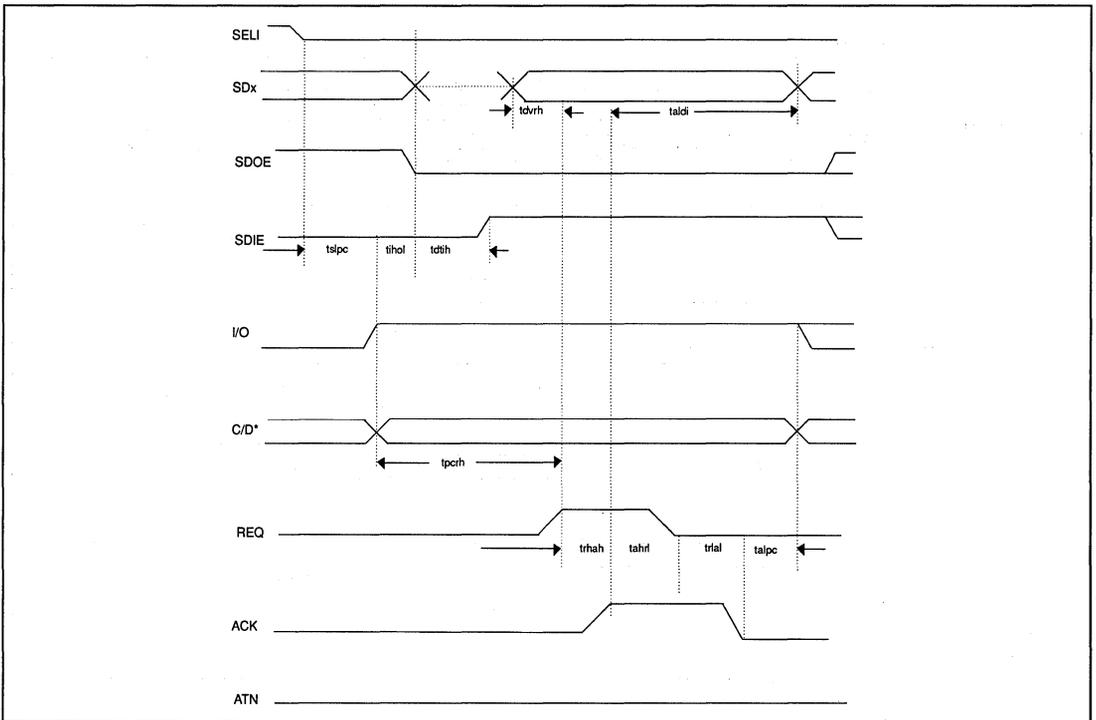
FIGURE 9-19. ASYNCHRONOUS INFORMATION TRANSFER IN(I)TIMING
