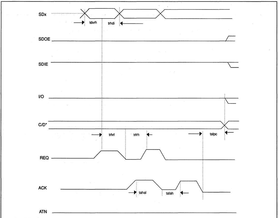
FIGURE 9-23. SYNCHRONOUS INFORMATION TRANSFER IN(I)TIMING
