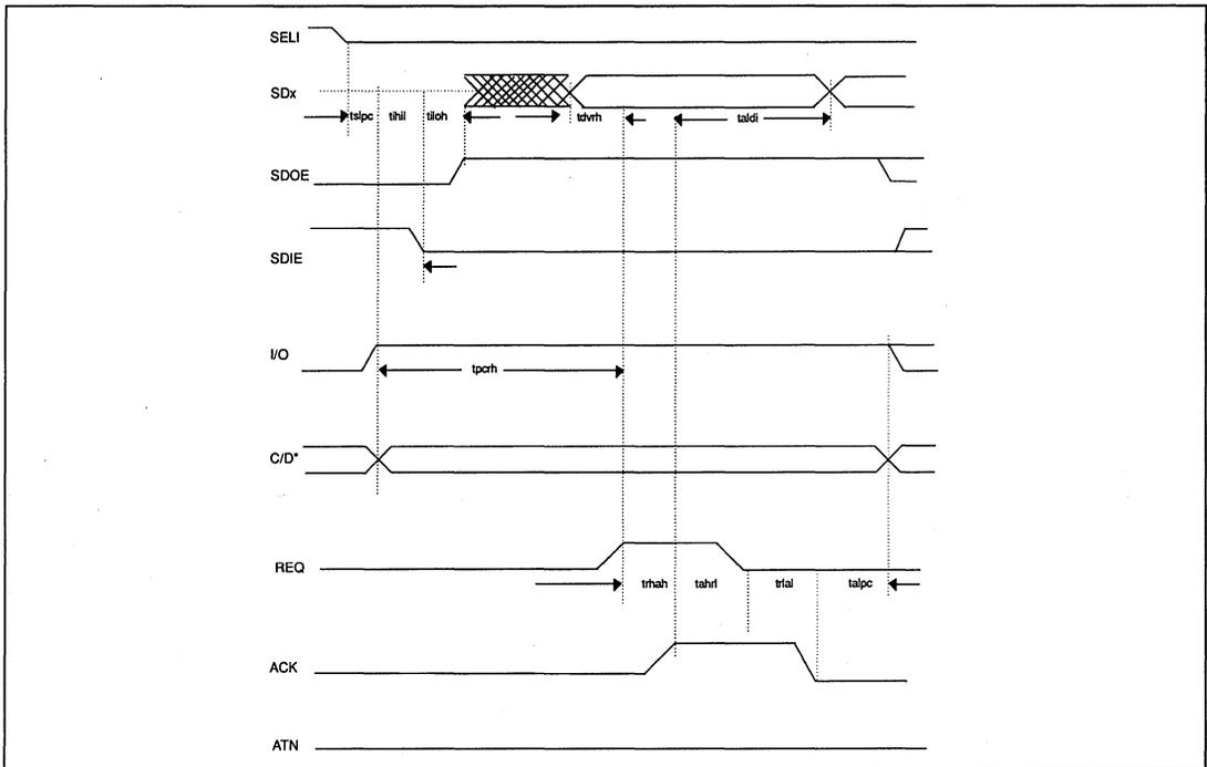
FIGURE 9-20. ASYNCHRONOUS INFORMATION TRANSFER IN(T)TIMING
