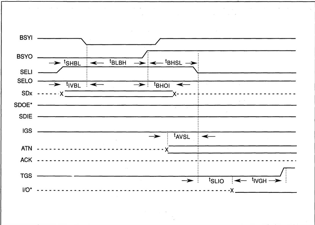
FIGURE 9-16. SELECTION (TARGET) TIMING
