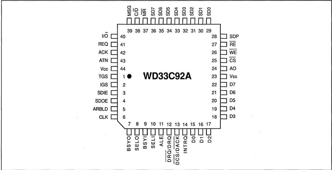
FIGURE 3-1. 44-PIN QUAD PIN DIAGRAM
