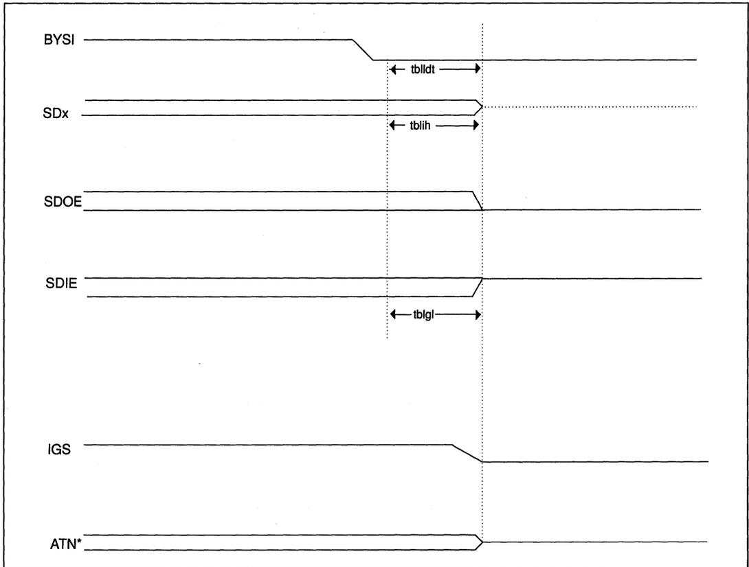
FIGURE 9-29. CONNECTED-AS AN-INITIATOR TO BUS FREE TIMING
