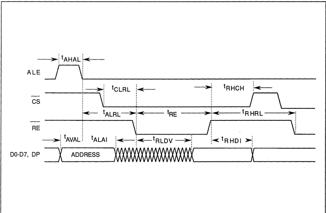
FIGURE 9-6. PROCESSOR READ (DIRECT ADDRESSING) TIMING
