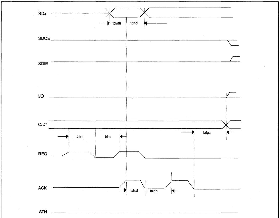
FIGURE 9-25. SYNCHRONOUS INFORMATION TRANSFER OUT(I)TIMING
