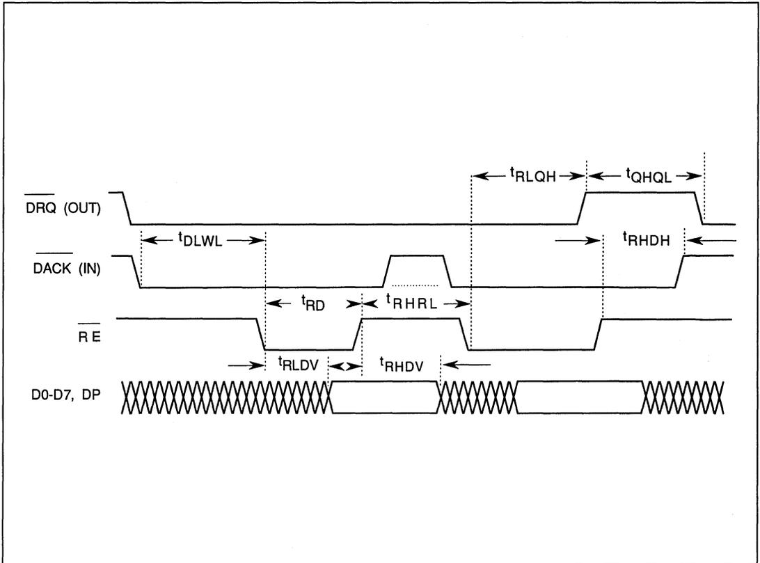
FIGURE 9-12. BURST DMA READ TIMING
