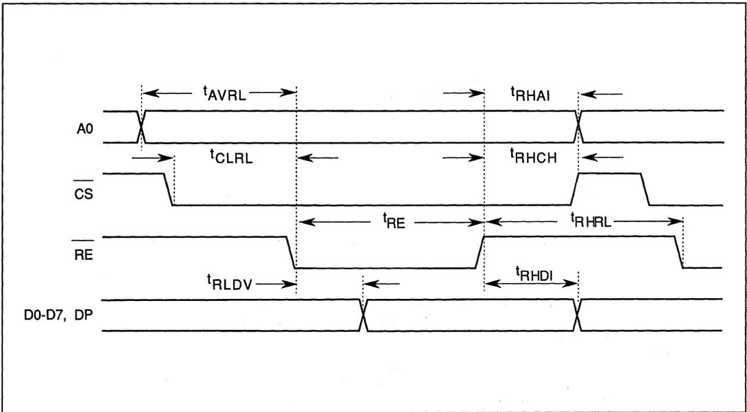
FIGURE 9-4. PROCESSOR READ (INDIRECT ADDRESSING) TIMING
