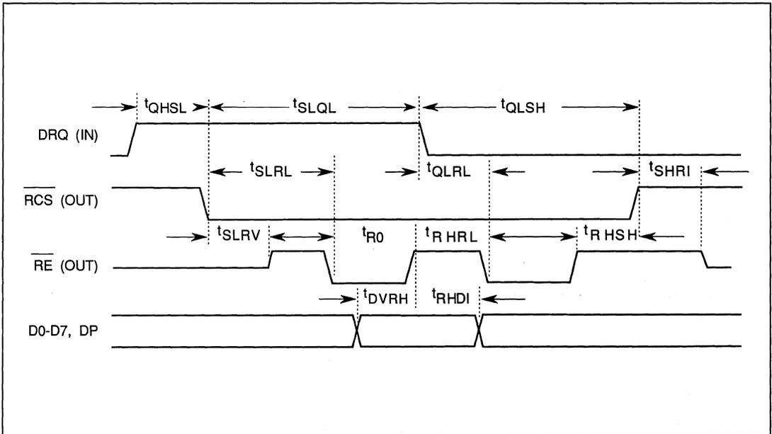
FIGURE 9-10. BUS BUFFER READ TIMING
