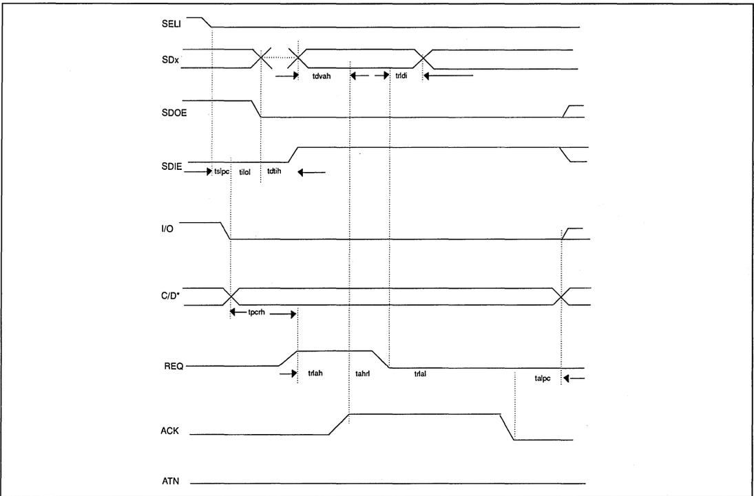
FIGURE 9-22. ASYNCHRONOUS INFORMATION TRANSFER OUT (T)
