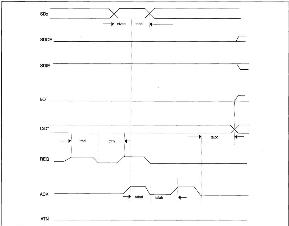
FIGURE 9-26. SYNCHRONOUS INFORMATION TRANSFER OUT(T)TIMING
