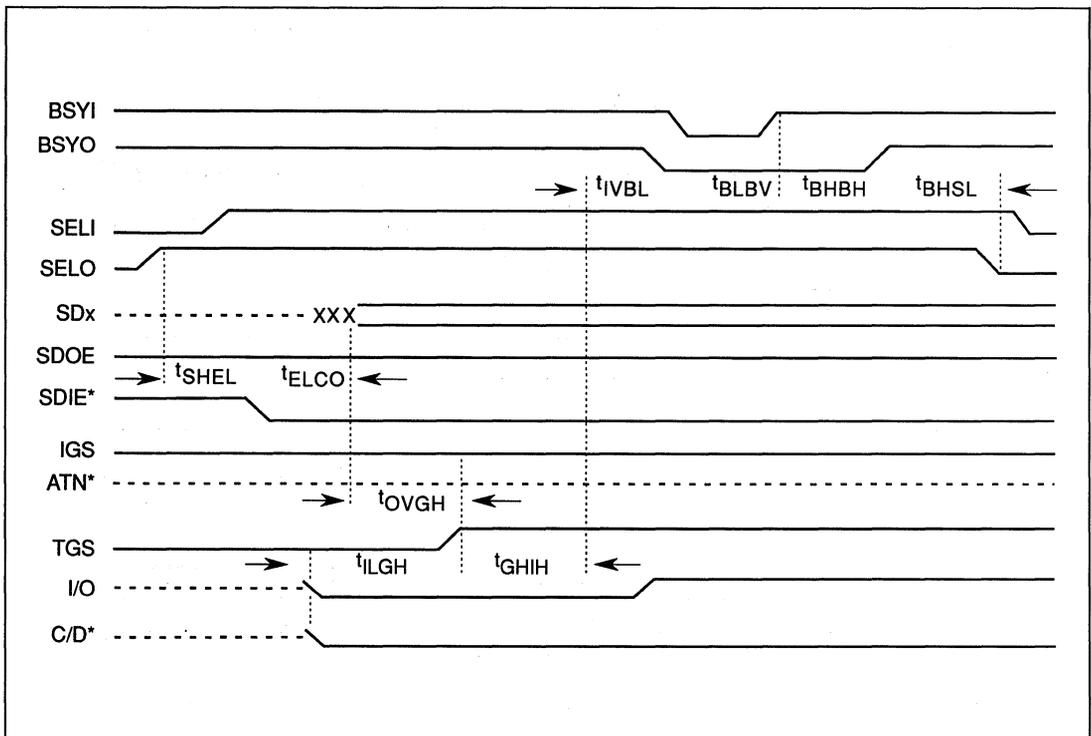
FIGURE 9-17. RESELECTION (TARGET) TIMING
