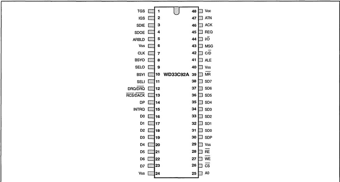
FIGURE 3-2. 48-PIN DIP PIN DIAGRAM
