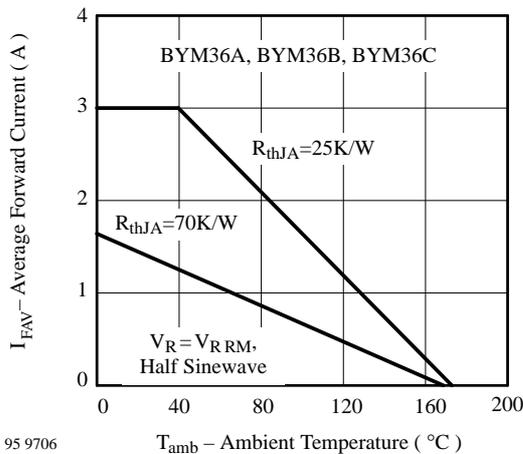
Figure 3. Average Forward Current vs. Ambient Temperature
