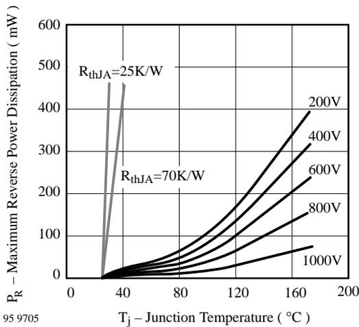
Figure 2. Maximum Reverse Power Dissipation vs. Junction Temperature
