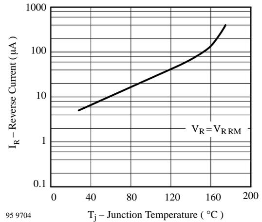
Figure 5. Reverse Current vs. Junction Temperature
