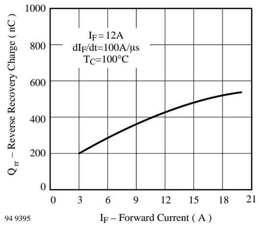
Figure 7. Reverse Recovery Charge vs. Forward Current
