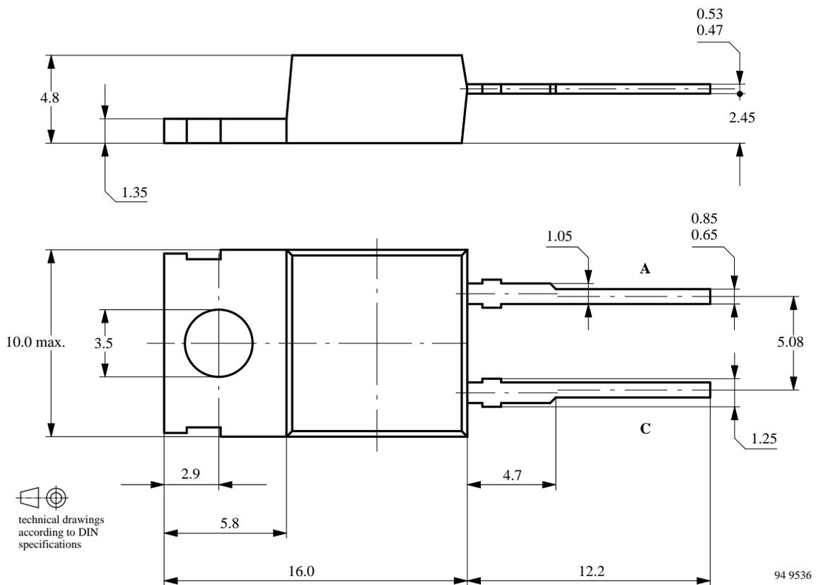
Cathode connected with metallic surface , Plastic Case DO 220 , Weight max.: 2.5 g
