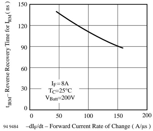
Figure 7. Reverse Recovery Time for I<sub>RM</sub> vs. Forward Current Rate of Change
