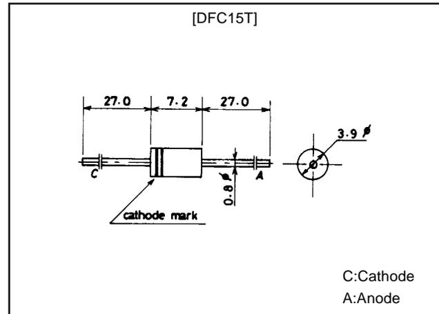
**Specifications****Absolute Maximum Ratings at  $T_a = 25^\circ\text{C}$**
