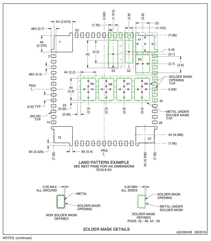
This package is designed to be soldered to the thermal pads on the board. For more information, see Texas Instruments literature number SLUA271 (www.ti.com/lit/slua271).
