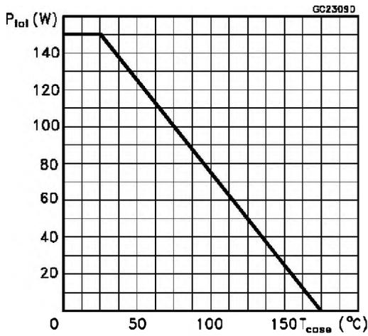
Derating Curve for ISOWATT220 Package
