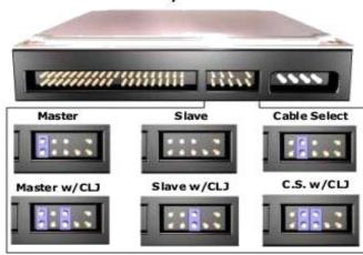
(Master) - The vertical jumper over the J50 pins is configuring the drive as a Master. The horizontal jumper over the J48 and J46 pins is in the Storage position.
